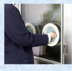
Can touch samples inside chamber without opening door. ( Up to 180°C)
